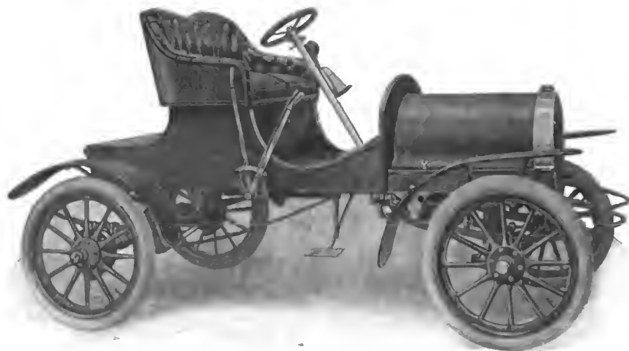
BATES 7-HORSEPOWER RUNABOUT WITH SINGLE-CYLINDER HORIZONTAL ENGINE.
